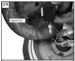
Remove the double sided tape from capacitor and stick capacitor to switch housing.
